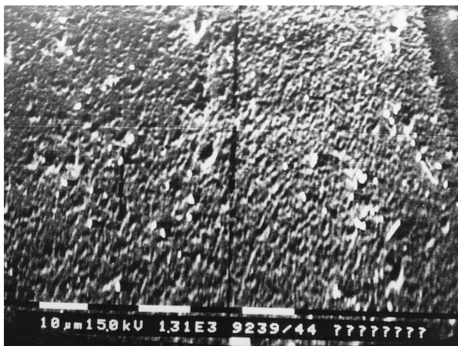
FIG. 7 Electron micrograph of CTA film treated in thiophene plasma for 20 minutes.
